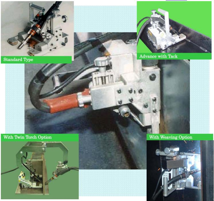
Light, compact, 4WD, and magnetic force traction with low center of gravity achieves highest pulling power and stability in the market. In addition, Vertical up position is possible.
